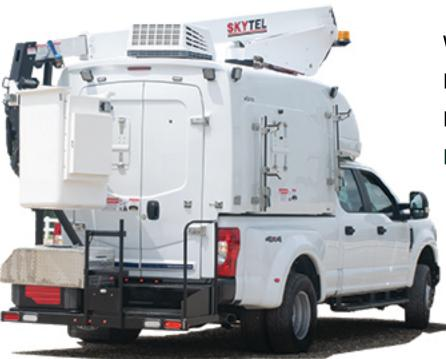
Working Height 34 ft 10 in (10.6m)\* Horizontal Reach 19 ft 6 in (5.9 m)\* Basket Capacity 350 lbs (159kg) Interior Height 6'2"
